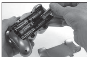
2. Insert 6 x 1.5 V AA batteries and observe the polarity information as shown in the battery compartment.
